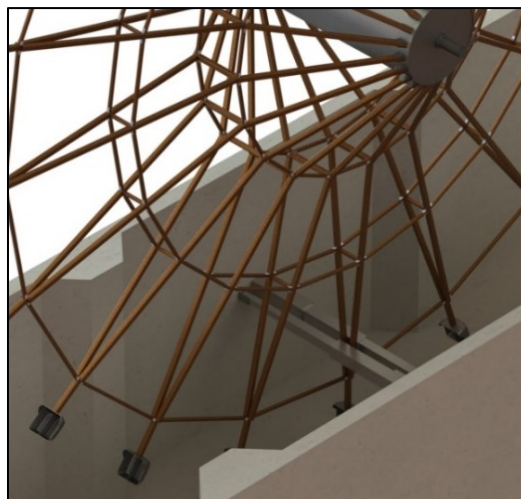
Figure 4-29: Possible Locking Mechanism - Locked Position
