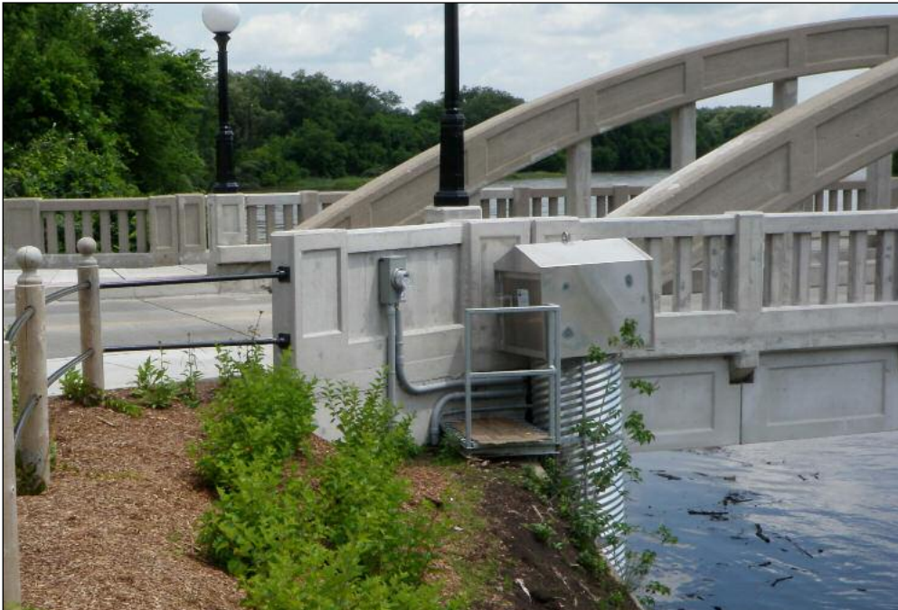
This flow gauge, located at Bridgeport Road in Kitchener, is one of 55 GRCA flow gauges used for flood forecasting and warning.
